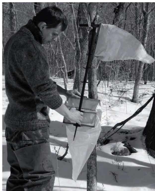
Fig. 2. Sampler preparation. Nets should be installed into CTNHs starting from the bottommost one.
